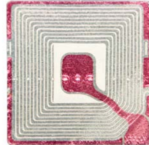
Typical RF Label Size is 1.5" L x 1.5" W
